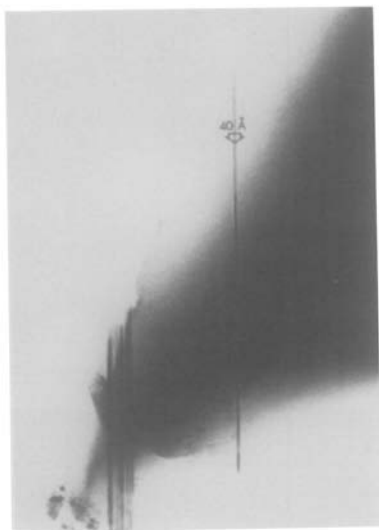
FIG. 6. Micrograph corresponding to Fig. 5. Groups of planar defects (twin planes) are more or less randomly distributed over the "MnS" matrix.
